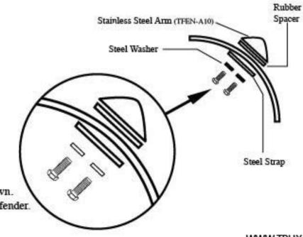
Place stainless steel arms to fenders as shown. Attach bolts with strap on the underside of fender.
