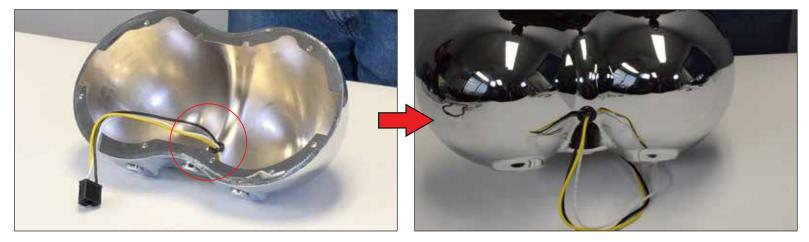
Place the *Gasket* on the *Housing Bucket* and feed the *Female H4 Connector* through the *Gasket*, making sure that the *Gasket* is in between the *H4 Connector* and the *Housing Bucket*.
