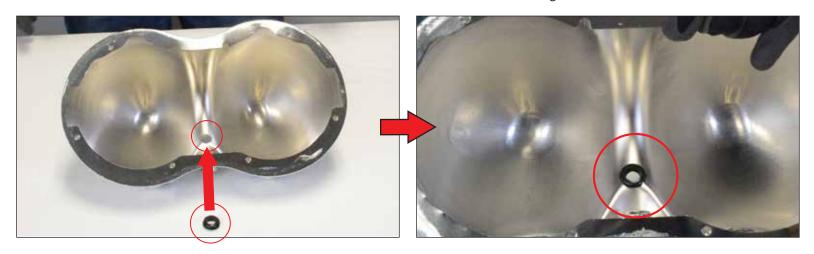
Feed the Yellow, Black and White Wires from the Female H4 Connector provided through the Black Rubber Grommet that is located in the center hole of the Housing Bucket. The Female H4 Connector should remain on the inside of the Housing Bucket.
