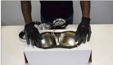
Without having any wires exposed, position the *Headlight Assembly* into the *Housing Bucket* and place onto the *Gasket*. Align the holes of the *Headlight Assembly* with the screw holes of the Gasket and the Housing.
