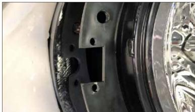
To secure the *Headlight Assembly* onto the *Housing Bucket*, place the provided *Screws* and *Washers* (see below for Washer order) into the screw holes located around the *Housing Bucket* (see below for locations). Using the provided *Phillips Screwdriver*, fasten all 6 screws to the *Headlight Assembly*.
