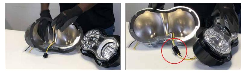
Connect the Headlight Assembly's Male H4 Connector to the Female H4 Connector found on the Housing Bucket.
