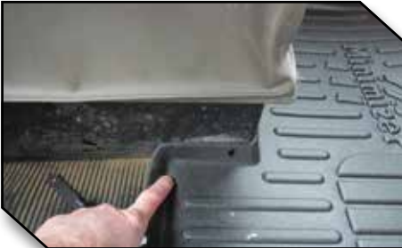
Figure 10 – Driver Mat Hook Location
