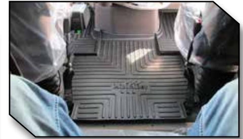
Figure 8 - Center Mat Installed
