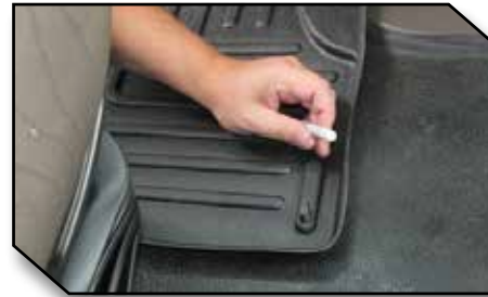
Figure 6 - Confirm Location Driver Mat and Hook
