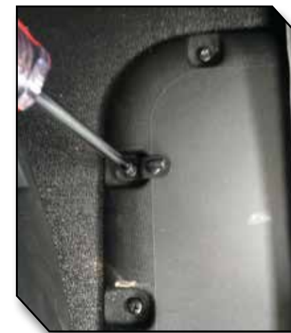
Figure 7 - Retention Hook Installation
