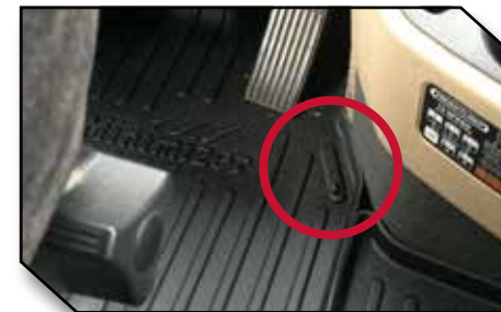
Figure 11 - Driver Mat Hook Installation
