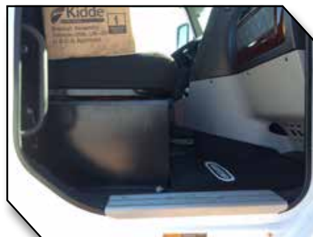
Figure 6 - Passenger Seat with Under Seat Battery Storage
