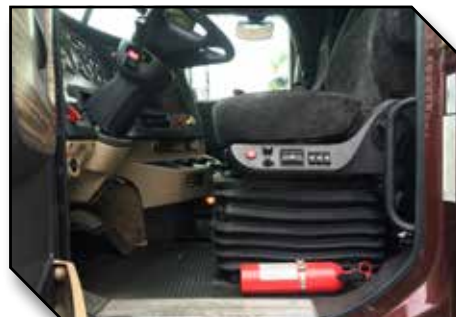
Figure 5 - Driver Seat with Rubber Skirt
