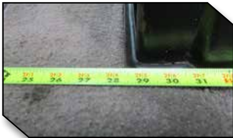
Figure 2 - 28.75” Measured at Front of Seat Base
