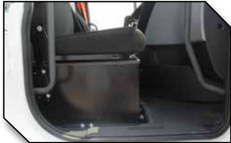
Figure 5 - Center Mat Trimming for Battery Box
