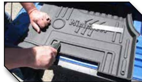
Figure 5 - Hand Trimming the Driver Mat for a Custom Seat Position
