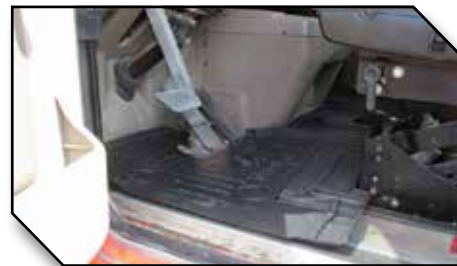
Figure 5 - Hand Trimming the Driver Mat for a Custom Seat Position
