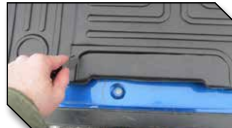
Figure 11 - Hand Trimming for Seat with Rubber Boot
