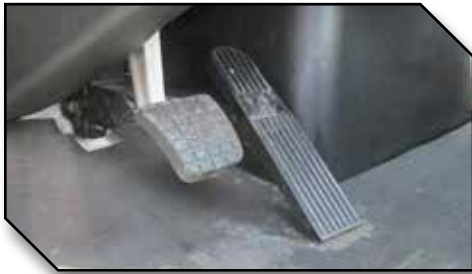
Figure 2 - Floor Mounted Throttle Pedal Mechanism
