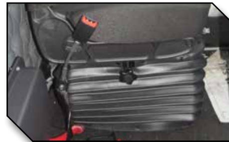
Figure 11 - Hand Trimming for Seat with Rubber Boot
