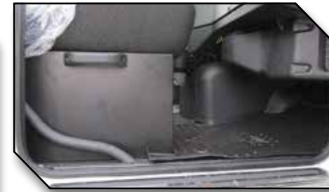
Figure 17 - Fixed Base Passenger Seat with Trimmed Mat
