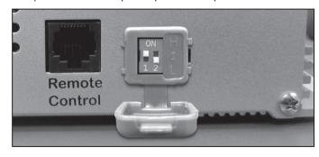
Note: Do not touch switch #1. It controls the inverter's *LVD\**UP: Alarm 11.5 V – Shutdown 11.0 V
