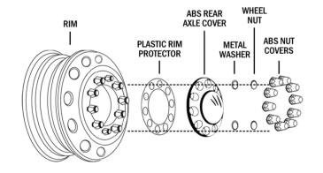
Threaded lug nut covers require a minimum of 1/2" of exposed thread.
