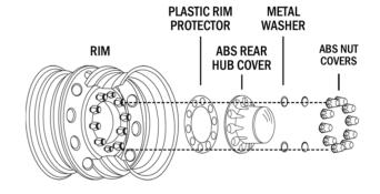
Threaded lug nut covers require a minimum of 1/2" of exposed thread.
