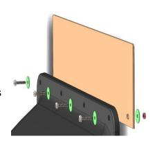
**2** Bolt the tubes to the quarter fenders using the hex head bolts, washers and **spring washers** as per diagram and tighten to 11 foot/pounds
