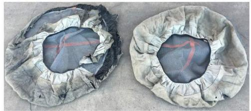
Obvious misuse of the product, where one sock is almost new and unused and the other sock is destroyed. Sock on the left is destroyed from uncontrolled spinning at full throttle.
